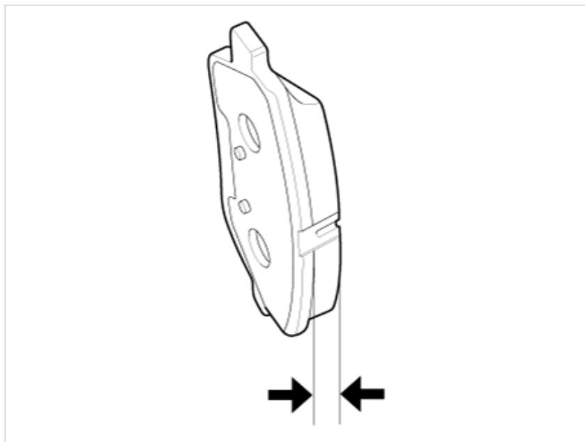
2. Check that grease is applied, to sliding contact points and the pad and backing metal for damage.
