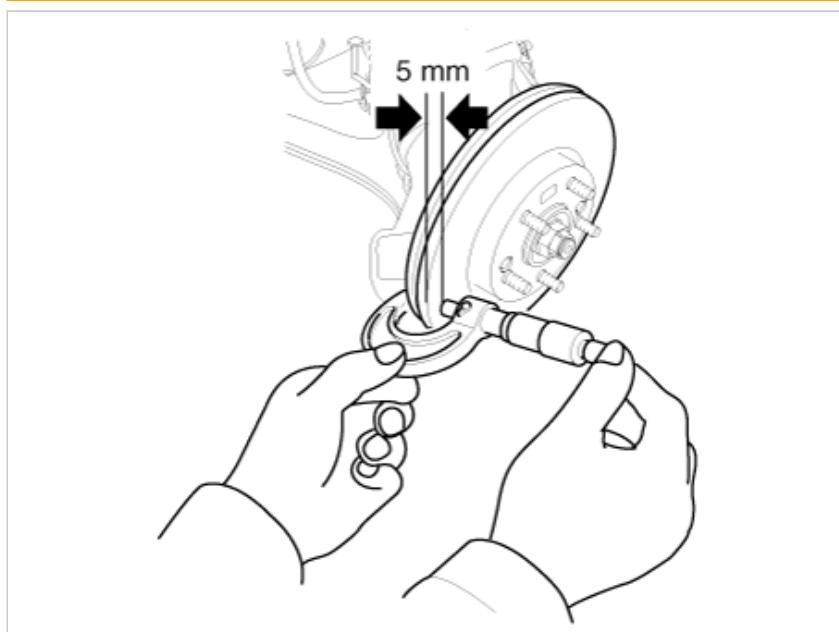
4. If wear exceeds the limit, replace the discs and pad assembly left and right of the vehicle.
