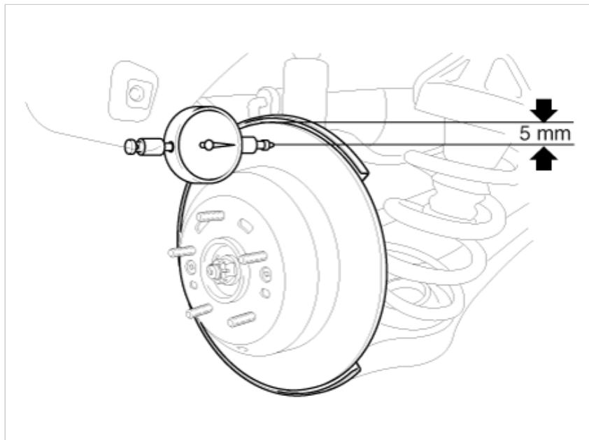
2. If the runout of the brake disc exceeds the limit specification, replace the disc, and then measure the runout again.
